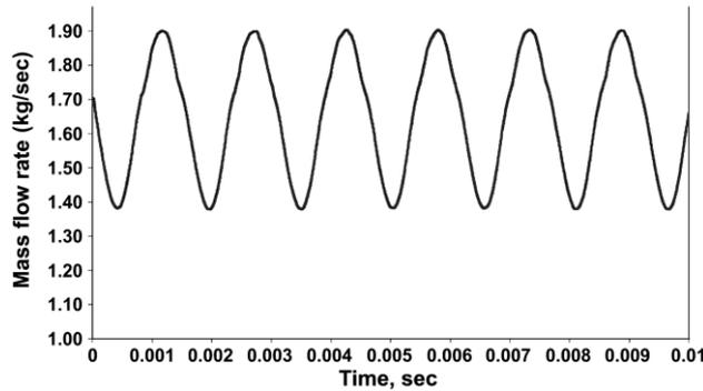
Fig. 1 – Mass flow rate curve in numerical modeling of a working fluid flow in the gear pump with the backlash of 30 μm, rotation frequency of 3000 rpm and pressure of 3000 psi (iteration step is 1 · 10<sup>-6</sup> s, the number of iterations is 10 000)
