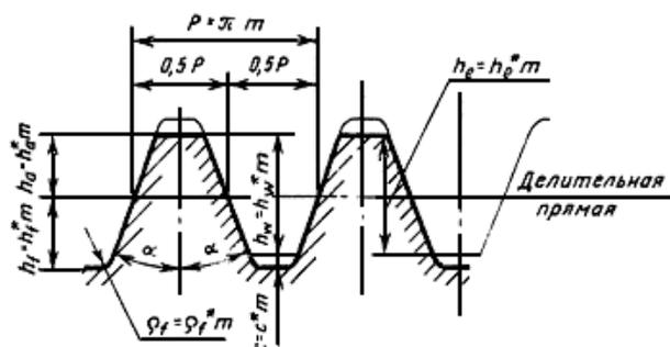
Fig. 2 – Theoretical basic rack profile of the tool (GOST 13755-81)
