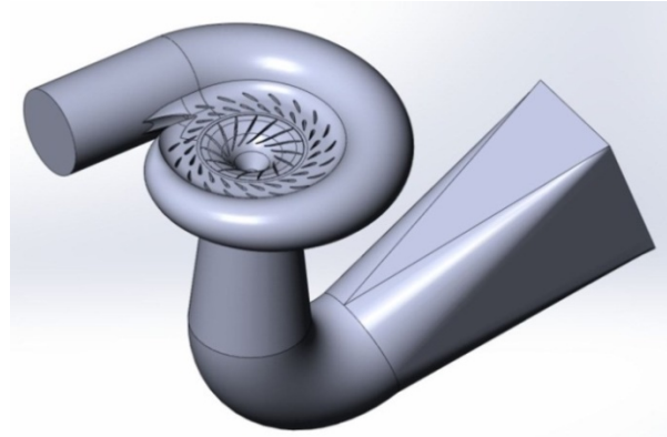
Fig. 1. Solid model of the flowing part of the hydro turbine Fr 310-V-100
