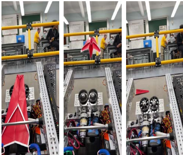
Fig. 2. Drone launch drive operation
